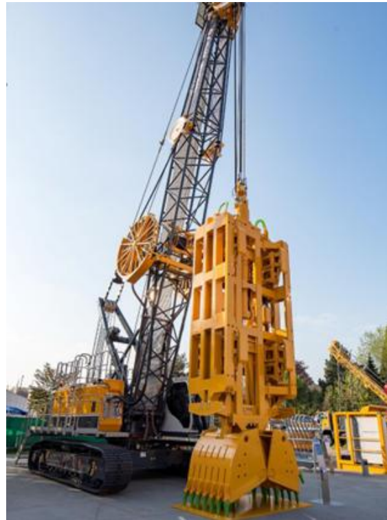
Fig. 2 Equipment for grabbed cut-off slurry wall (1).
