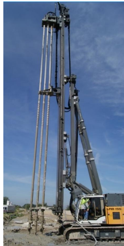
Fig. 7 Equipment for DSM technology – multiple mixing tools (12).
