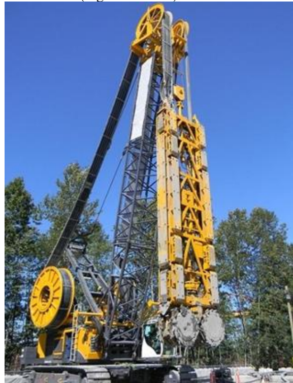
Fig. 3 Cutter soil mixing with mixing tools rotating about horizontal axes (1).
